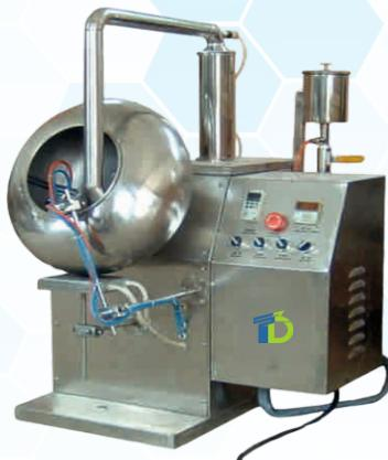
Conventional Coating Pan is made after a careful study of needs of expert coaters such as Rotation Speed, Angle of Pan, volume and temperature. It is elliptical in shape, mounted at 30° angle. Hot air blower thermostat of the pan delivers required quantity of air at selected temperature between 40°C to 80°C
