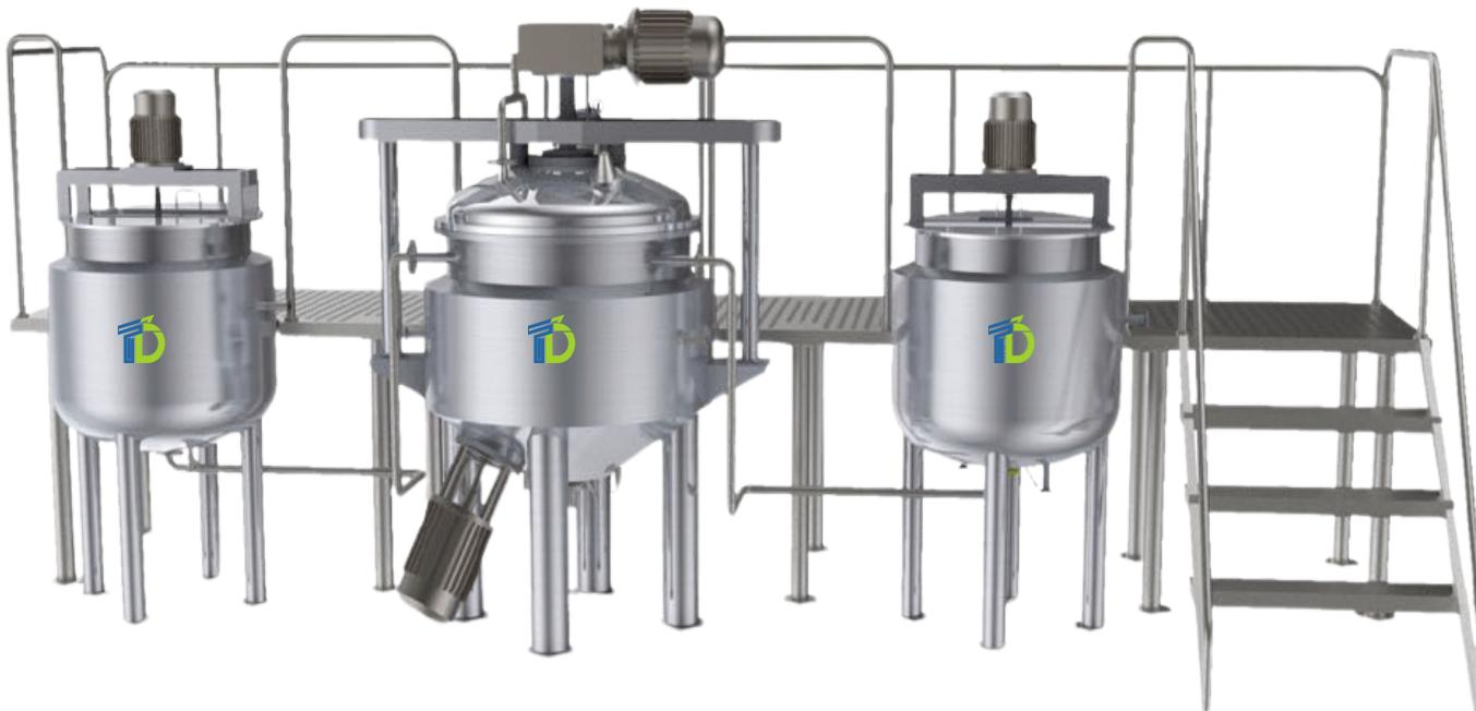
The Ointment Manufacturing Plant consists of a set of equipment designed for ointments ranging from 5 kg to 5,000 kg. They are excellent devices for the pharmaceutical and cosmetic industries.
